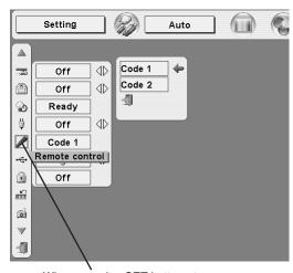
When pressing SET button at Remote control, Remote control code Menu appears.
